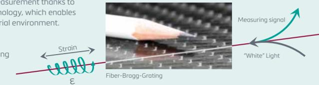
our fiber-optic sensors and technology for rotor blades, which can withstand 1000 times more load reversals at up to 10 times higher amplitudes when compared to electrical measurement technology.
